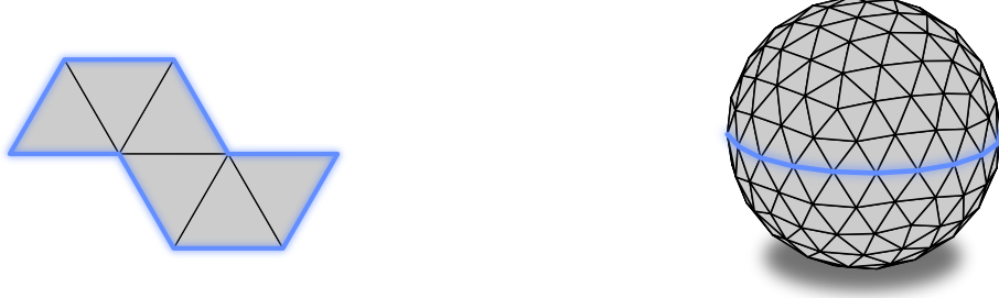
Figure 5: Left: The cycle \gamma is the blue boundary with \pm 1 coefficients, and the unique unit \gamma -flow is the 6 triangles in series. If the complex is unweighted, then the effective resistance of \gamma is 6. Right: The cycle \gamma is the equator of the sphere, and the two hemispheres are two unit \gamma -flows in parallel. If each hemisphere has flow energy c , then the effective resistance of \gamma is \frac{c}{2} .
